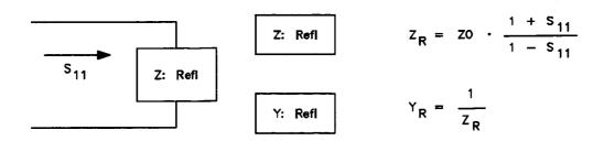
Figure 5-5. Reflection Impedance and Admittance Conversions
