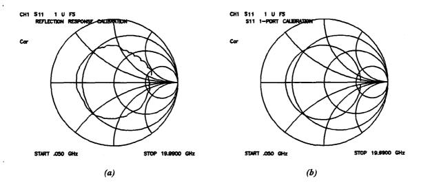
Figure 6-5. Response vs. S11 1-Port Calibration on Smith Chart
