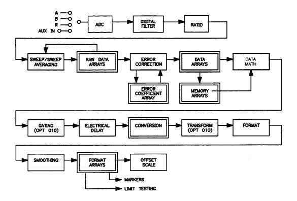
Figure 2-2. Data Processing Flow Diagram
