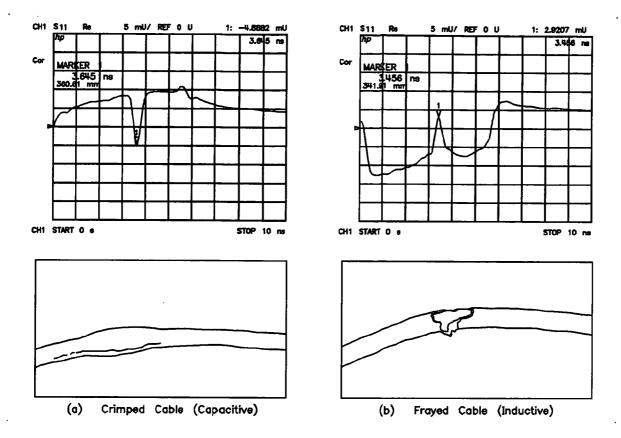
Figure 9-7 shows example cables with discontinuities (faults) using the low pass step mode with the real format.
