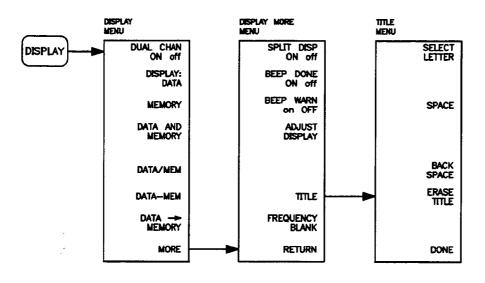
Figure 5–23. Softkey Menus Accessed from the DISPLAY Key
