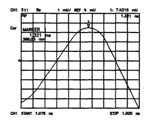
Figure 9–13. Range Resolution of a Single Discontinuity
