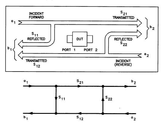
Figure 5-3. S-Parameters of a Two-Port Device
