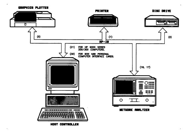
Figure 12–2. Analyzer Single Bus Concept
