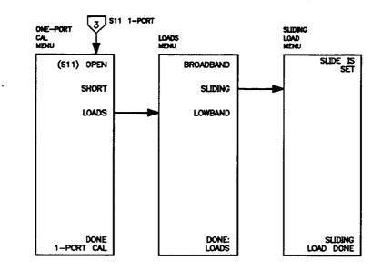
Figure 6-15. Menus for S11 1-Port Calibration
