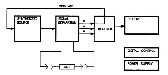
Figure 2-1. Simplified Block Diagram of the Network Analyzer
