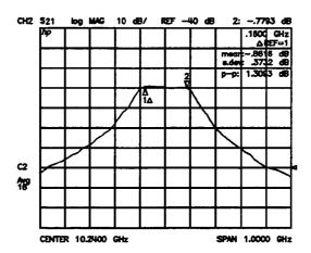
Figure 7–12. Measurement Using Marker Statistics
