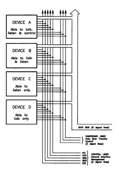
Figure 12–1. HP–IB Structure
