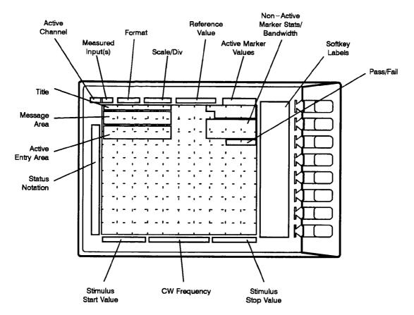
Figure 3-4. CRT Display (Single Channel, Cartesian Format)
