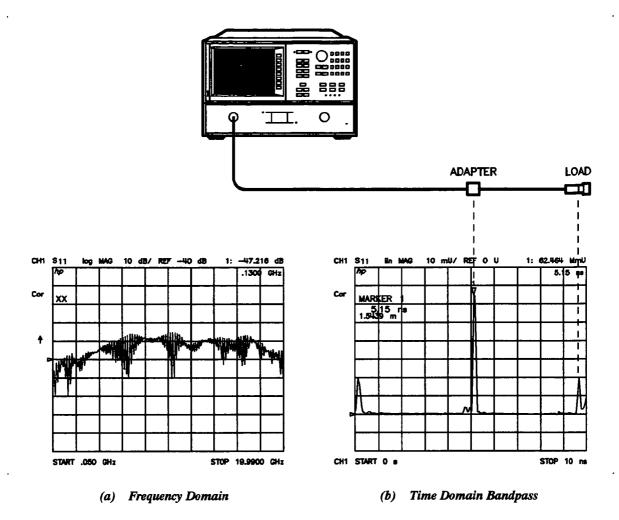
Figure 9-3. A Reflection Measurement of Two Cables
