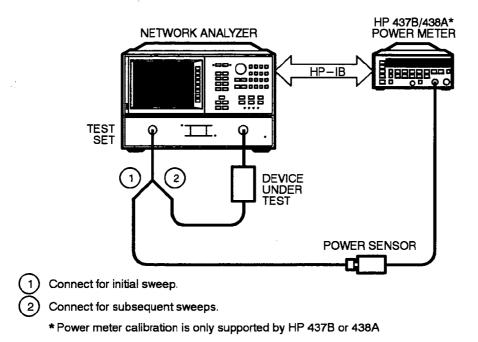
Figure 6-18. Typical Test Setup for Sample-and-Sweep Correction
