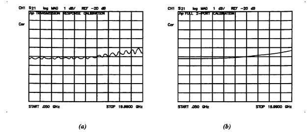
Figure 6-6. Response vs. Full Two-Port Calibration
