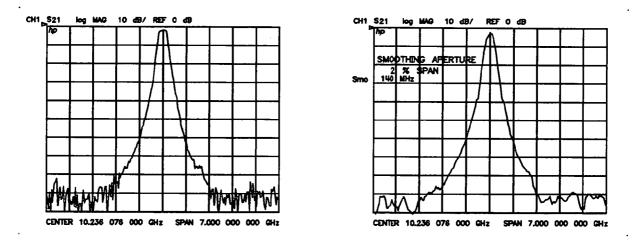
Figure 5-32. Effect of Smoothing on a Trace
