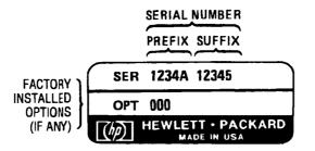
Figure 1-2. Typical Serial Number Plate
