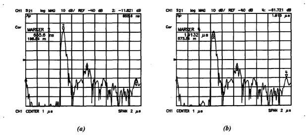
Figure 9-4. Transmission Measurement in Time Domain Bandpass Mode
