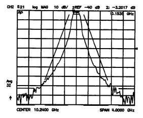
Figure 8–6. Limit Lines for Bandpass Filter Testing
