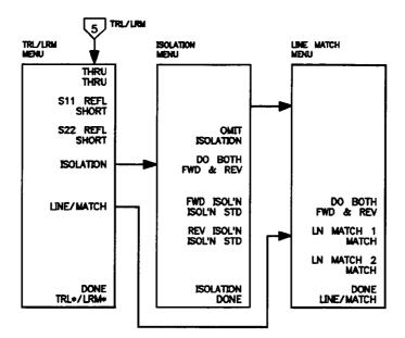
Figure 6-17. Menus for a full 2-Port TRL/LRM Calibration
