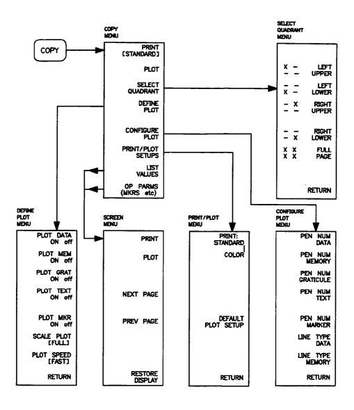
Figure 10-1. Softkey Menus Accessed from the COPY Key
