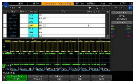
Figure 15. I 2 C decode and trigger.
