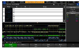
Figure 16. RS232 decode and trigger.
