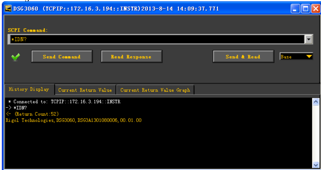
Figure 3-5 Write and read commands via LAN
